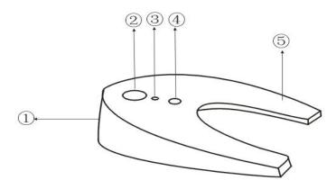
① 48V phantom power connection cable port (6 meters shielded cable,
